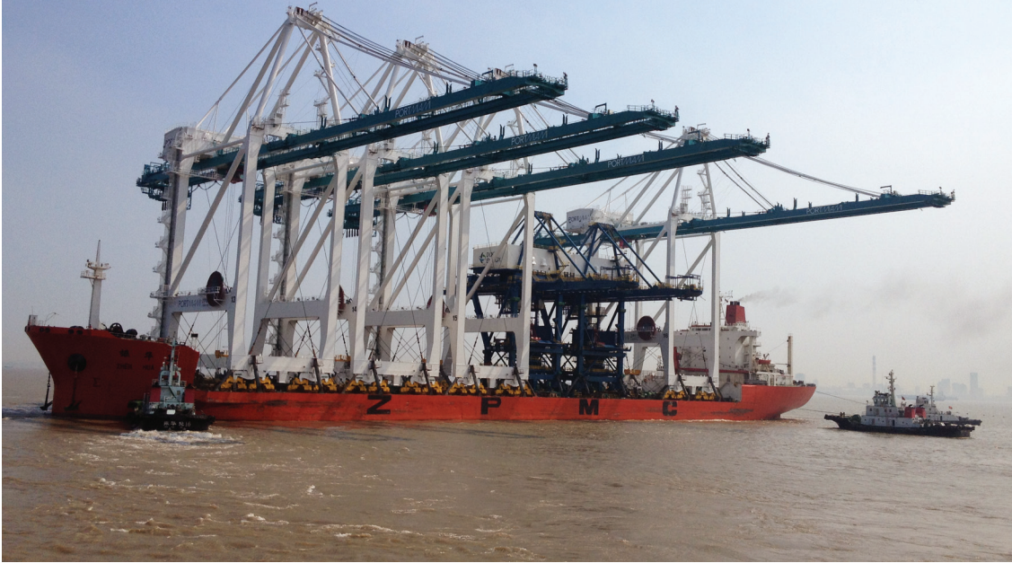
Four new super-post-Panamax cranes make the waterborne journey to PortMiami from China.
